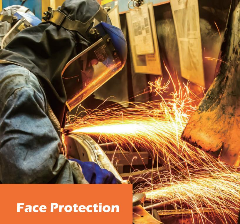
The faceshield can be used to provide all-round protection for the face and eyes of the wearer in the work environment.
